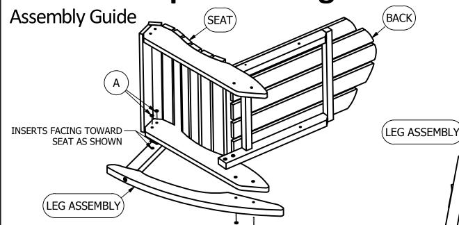
**3)** Attach Front of Leg Assembly to Seat Using Two "A" Bolts as Shown Above. Attach Back of Leg Assembly to Seat Using Two "B" Bolts as Shown Below.
